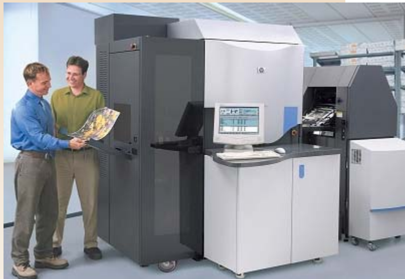
HP Indigo 3050 liquid EP press - 11"x17", 7-color, 2K sheets/hr. 4-color) (67 8.5"x11" ppm)
