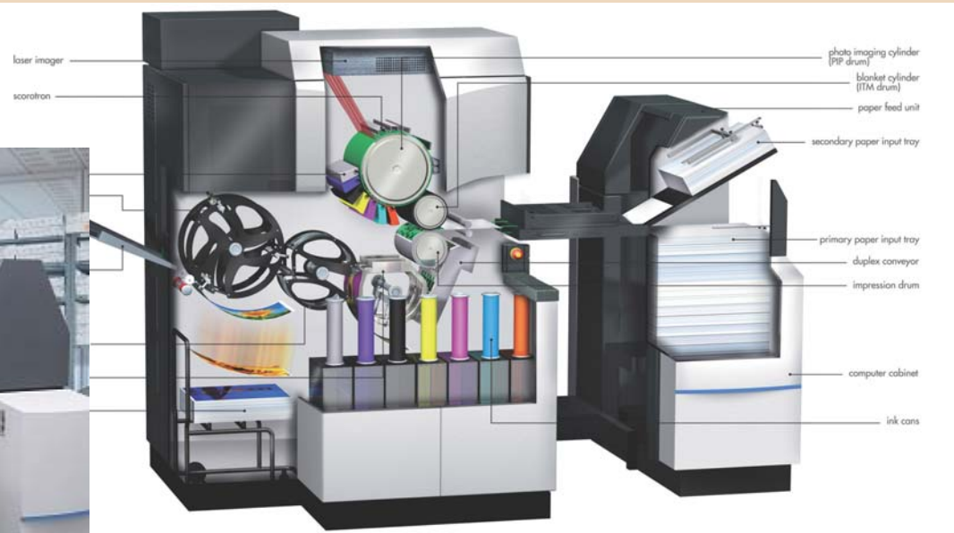
HP Indigo 3050 liquid EP press - 11"x17", 7-color, 2K sheets/hr. 4-color) (67 8.5"x11" ppm)
