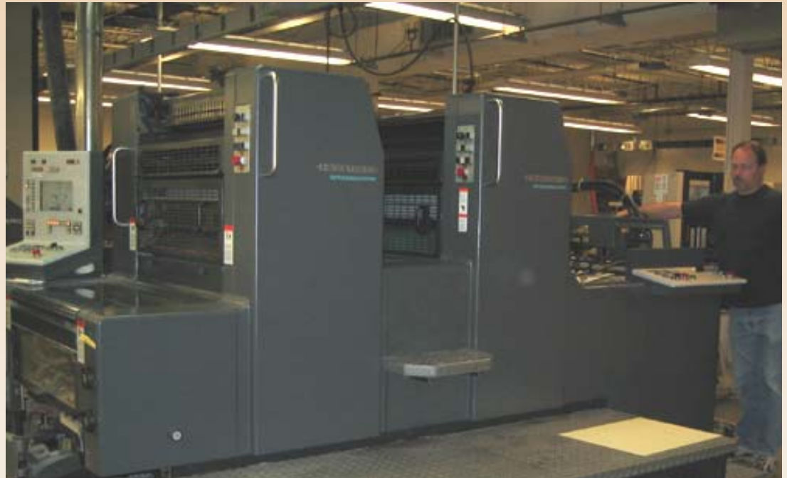
Heidelberg Speedmaster SM 74 offset press 20"x29", 2-color, 10K sheets/hr.
